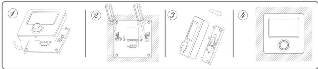
Step 1: Carefully separate the front half from the back plate.
