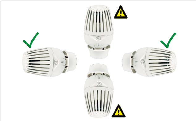
**⚠** These positions are not recommended due to the influence of the radiator temperature on the thermostatic head.
