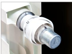
**4)** After the limiters have been positioned, return the knob to the initial adjustment position (3), applying sufficient pressure.
