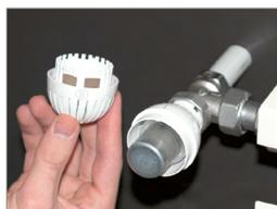
**3b)** In order to **lock** the adjustment range, position a limiter to the right of the number corresponding to the maximum desired opening and a limiter to the left of the number corresponding to the minimum desired opening. This prevents the head from being either opened or closed.
